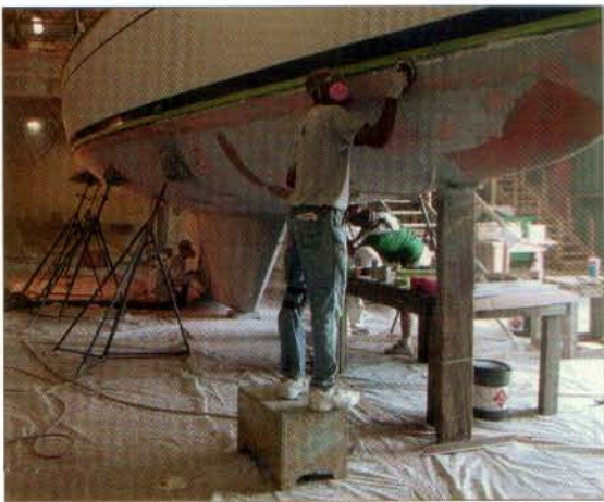
Top —The bottom was faired with vinyl ester putty after laminating. Bottom —Bottom paint was applied with an airless sprayer.
